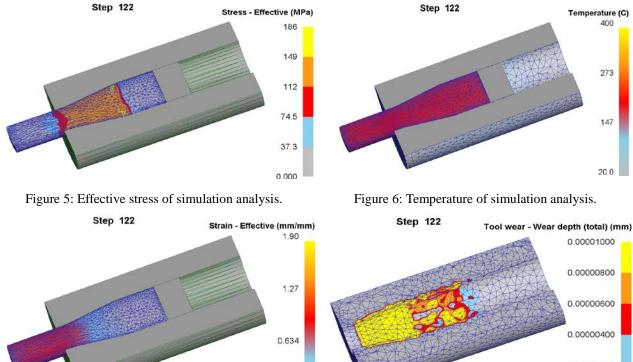
Figure 7: Strain effective of billets extruded.
