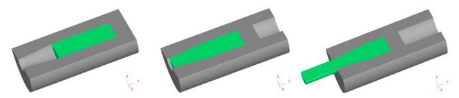
Figure 4: Simulation analysis of an extrusion die process; a) before extrusion; b) middle extrusion; and c) after extrusion.
