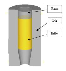
Figure 2: Extrusion die designed.
